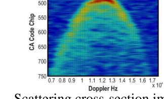
Scattering cross-section image measured by UK-DMC-1 spaceborne mission with variable lag correlation and Doppler shift
